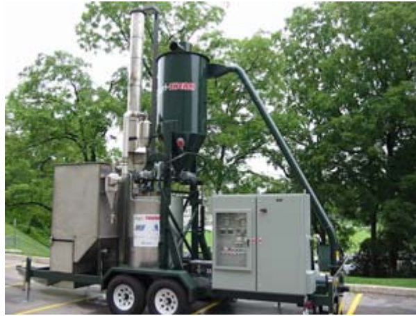
Figure 3-4 Agri-Therm portable fast pyrolysis unit (Agri-Therm, 2011)
